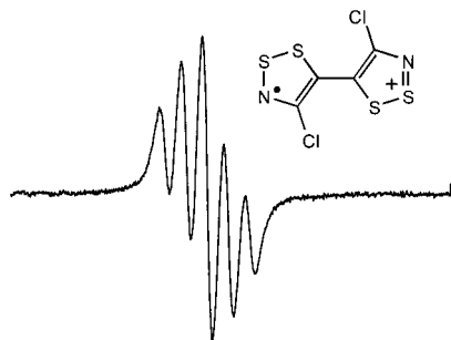
Figure 2. X-band ESR spectrum of [DC-TAF][ClO 4 ] in SO 2 (l). Sweep width = 2 mT.
